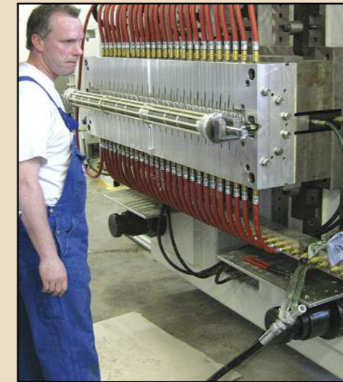
Primed module inserted into mold.
