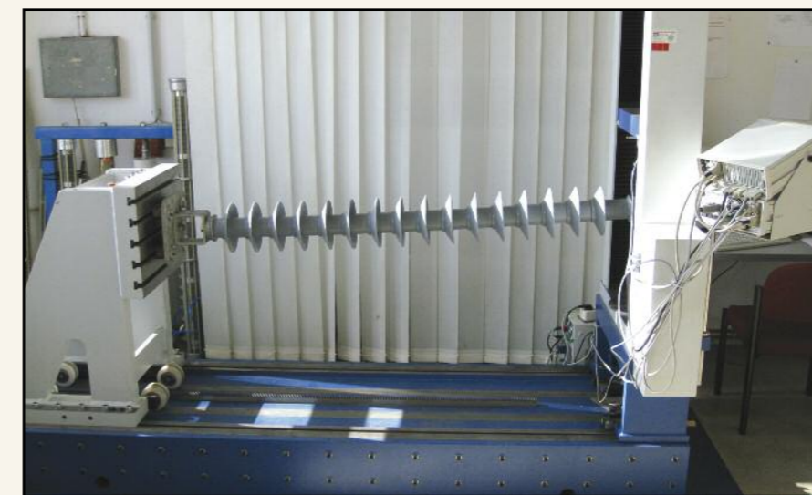
Wrap design polymeric arrester being tested for bending load.
