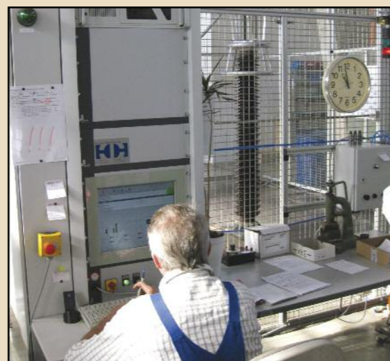
In process test field equipped with all new instrumentation automatically links test results with all production data.
