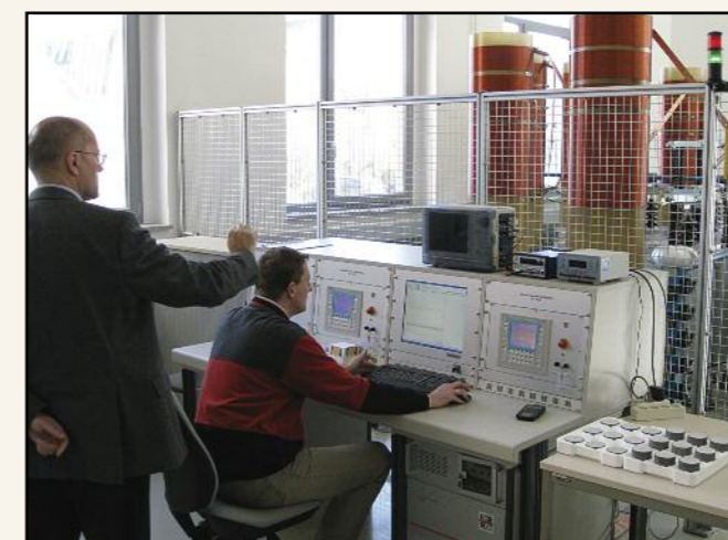
New test field for verifying quality of incoming varistor blocks allows graphical representation of results (right).
