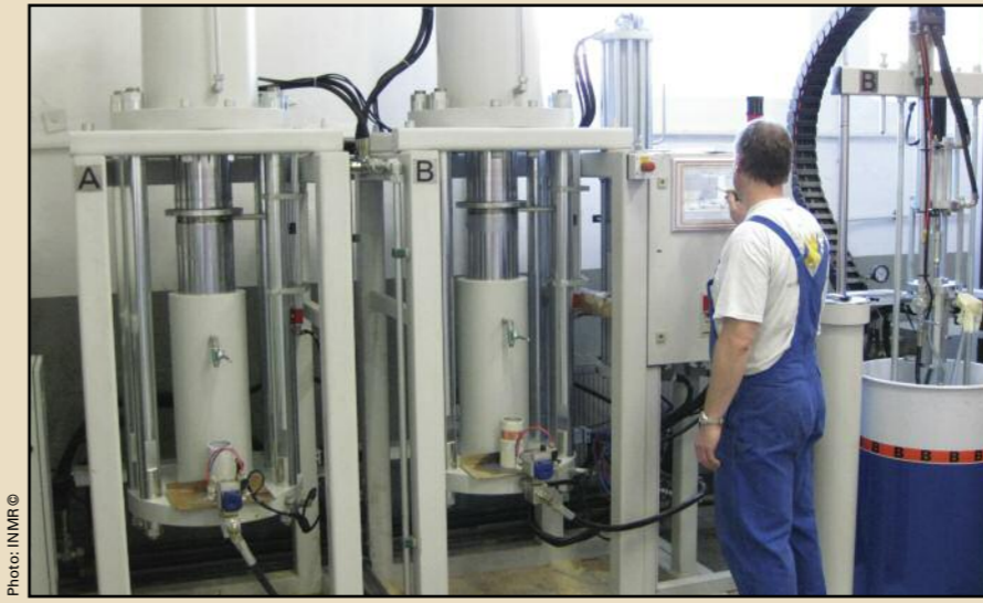
Liquid silicone rubber in two-component system is dosed to static mixer before being pumped into mold cavity.
