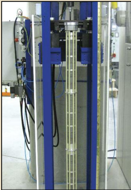
Machine attaches end fittings and transfers tensile load to rods to yield mechanical strength of caged module.
