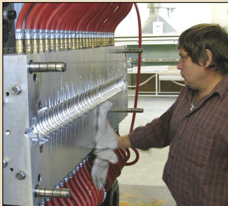
Cleaning mold cavities prior to start of next curing cycle.
