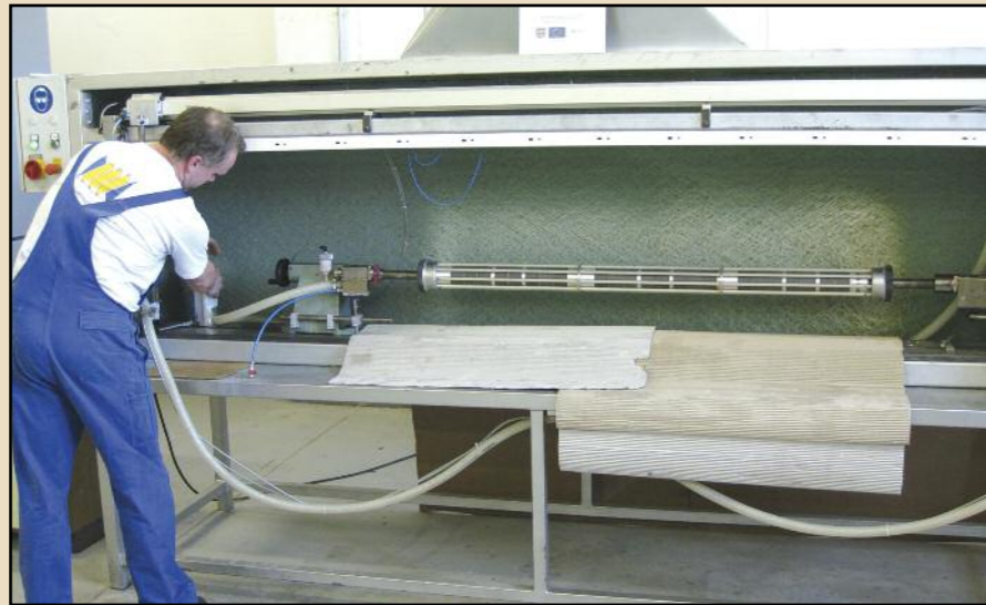
Drying of cleaned caged module prior to priming
