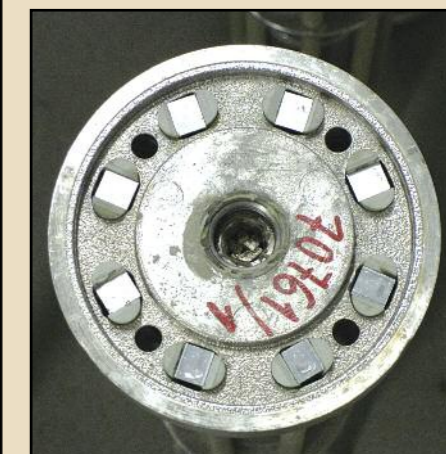
Wedges are driven into notches in fiberglass rods to complete cage around varistor blocks.
