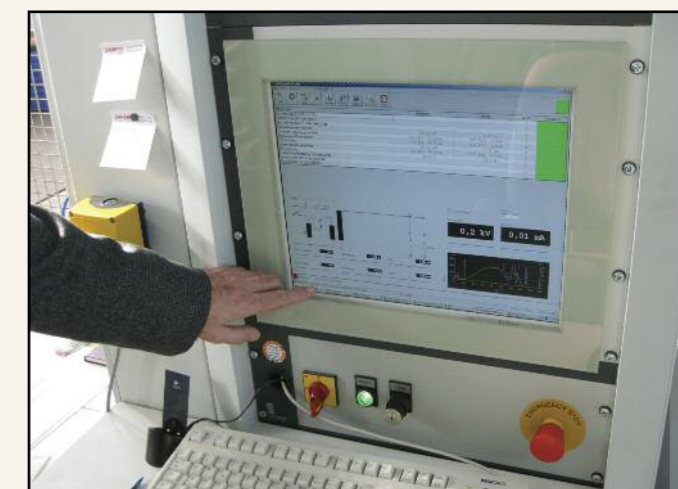
New test field for verifying quality of incoming varistor blocks allows graphical representation of results (right).
