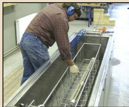
Drying of cleaned caged module prior to priming
