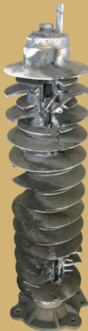
Cage design demonstrates safe failure mode after 63 kA short circuit for 0.2 seconds.
