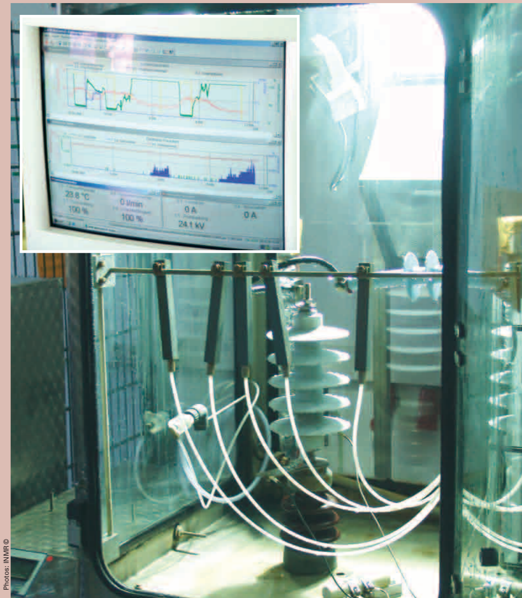
Key parameters measured (inset) as 24 kV arrester undergoes 5000-hour accelerated ageing.
