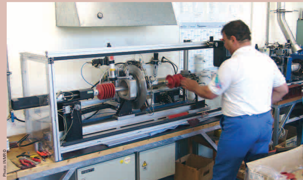
Machine allows for flexibility in determining number and spacing of sheds along the arrester.
