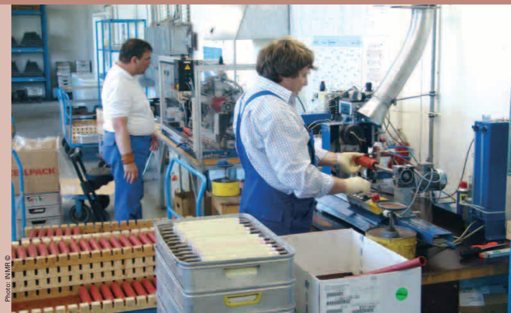
Cured moules (foreground) inserted into silicone tubes under vacuum.
