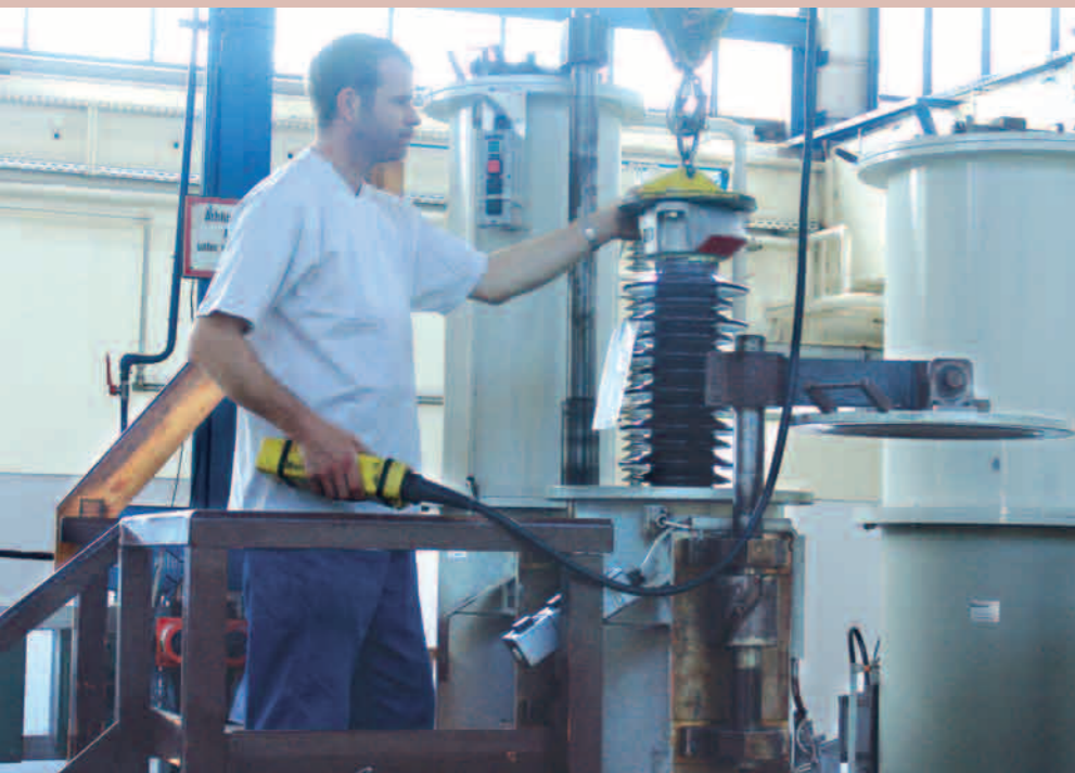
Sealed arrester placed into vacuum chamber to detect presence of any escaped helium gas.
