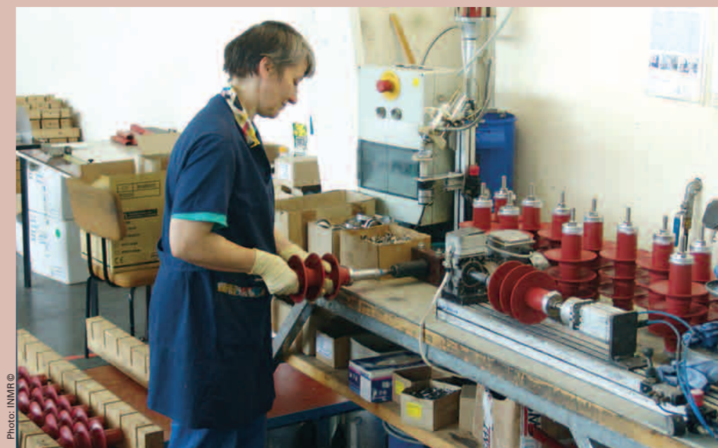
Installation of end fittings onto MV wrapped type arresters.
